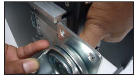
Quick Release Wheels with Safety Lock
