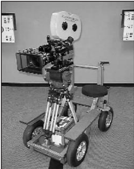
Action Dolly equipped with tripod
